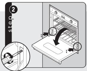
Open door completely. Reinstall hinge trim plates.
